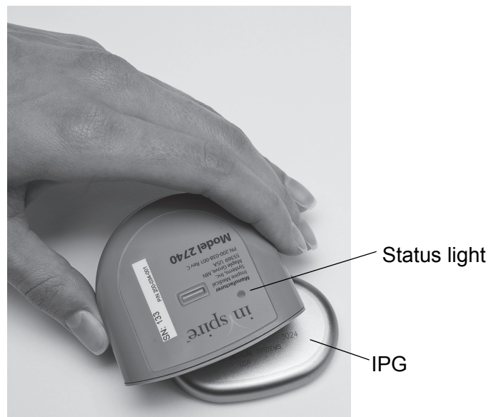
Figure 3-7. Correct Positioning of Telemetry Head over IPG
