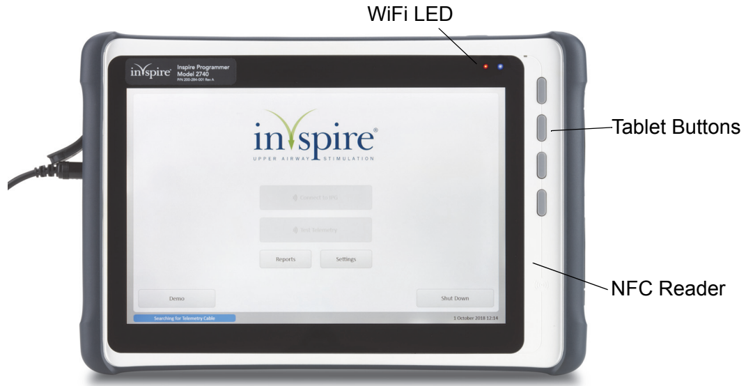
Figure 8-1. Unused Tablet Features, Front
