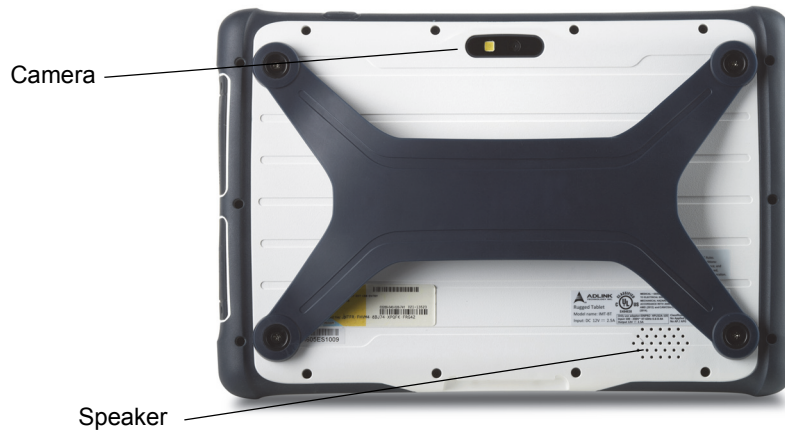
Figure 8-4. Unused Tablet Features, Back
