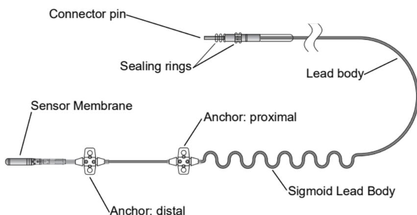
Figure 1. Respiratory sensing lead
