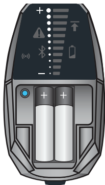
Figure 17. Battery compartment and battery placement
