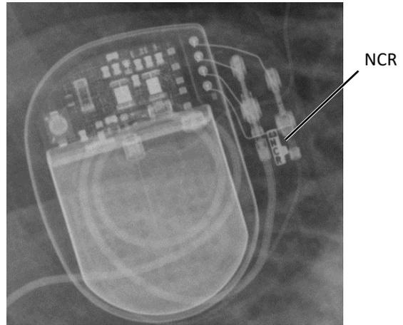
Model 3024: X-ray ID is "NCR" and generator is not eligible for an MRI
