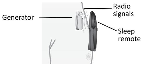
**Figure 4.** Communication between sleep remote and generator
