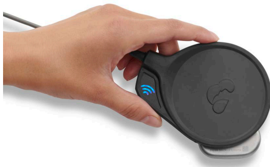
Figure 4-3. Correct Positioning of Programmer Head over Generator
