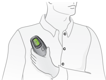
Figure 4-9. Correct positioning of sleep remote over generator
