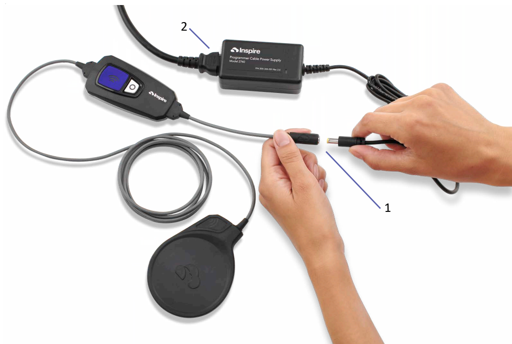
Figure 4-2. Programmer Cable Power Supply Connections
