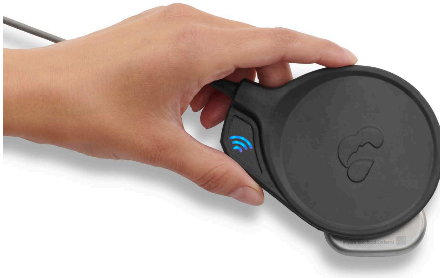
Figure 4-3. Correct Positioning of Programmer Head over Generator
