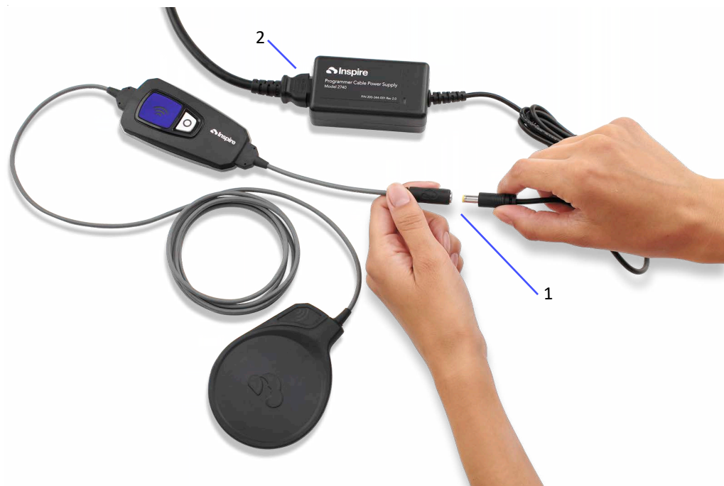
Figure 4-2. Programmer Cable Power Supply Connections
