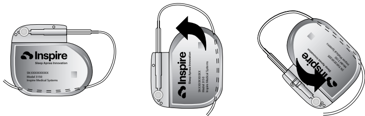
Figure 13. Wrap excess lead length
