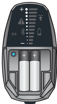
Figure 6-2. Battery compartment and battery placement
